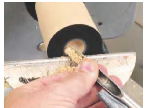
▲ Pic.14 Once the gouge has drilled a small hole in the centre, it is pivoted out by moving the handle away from the body
